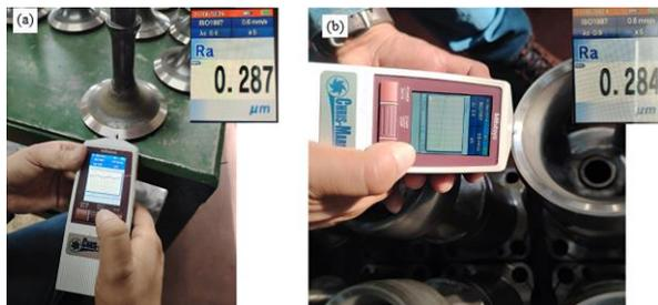
Figure 13: (a) Measurement of the roughness in the exhaust valve. (b) Measurement of the roughness in the exhaust box.
