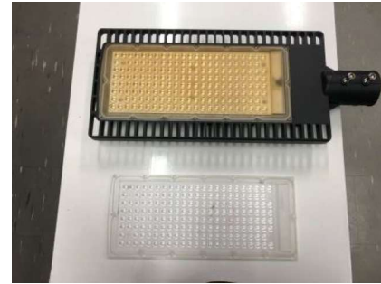
Figure 7: The 150W Luminaire Recorded Before and After Six Thousand Hours of Exposure
